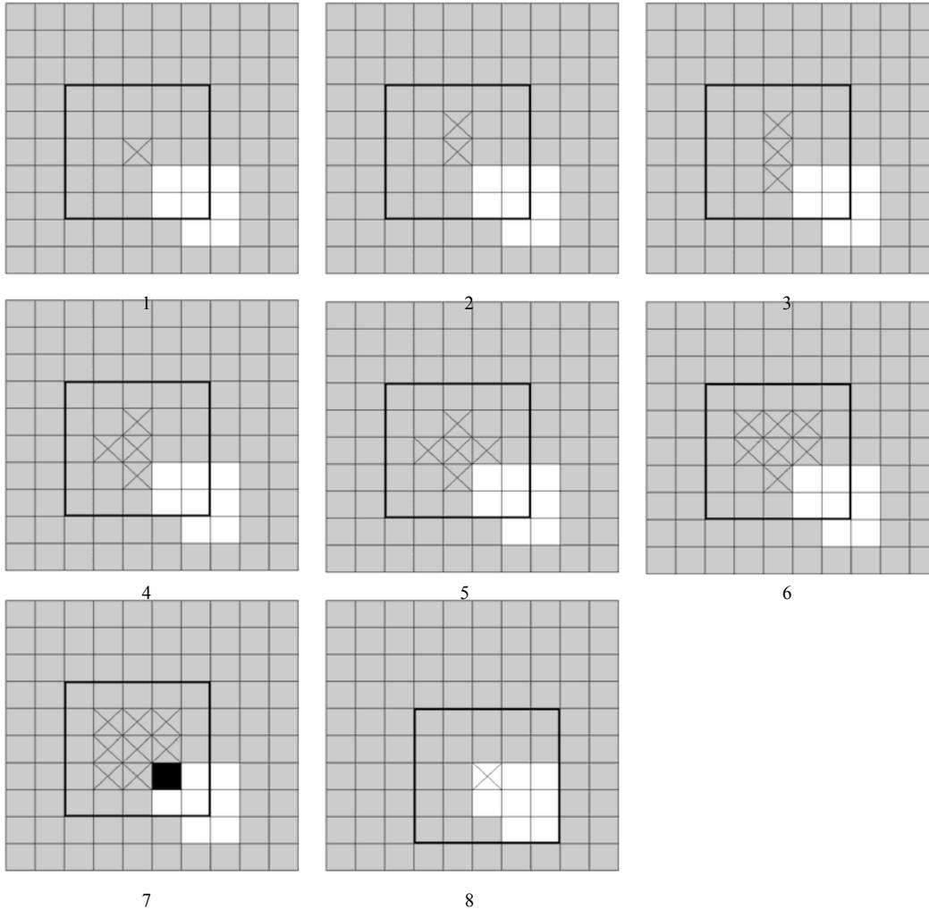
Fig. 3 Bacterium search algorithm. Grids 1 to 5 present the process of one loop of the tracking procedure. The second loop starts on grid 6 and ends on grid 7 when a bacterium is found. Search area center is adjusted and the first part (Fig.2) of the algorithm is then launched.
