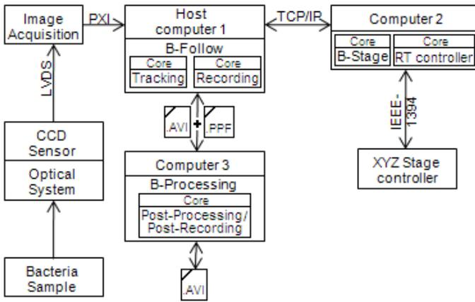
Figure 2. Data flow interconnections showing the multi computers architecture
