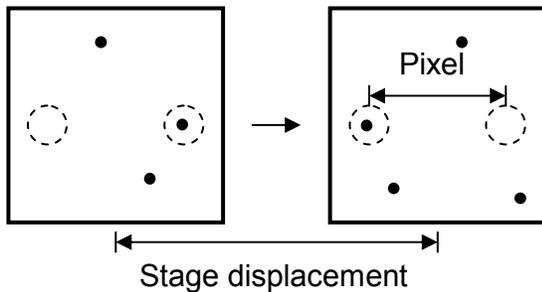
Figure 4. Micrometers to pixels ratio calibration algorithm
