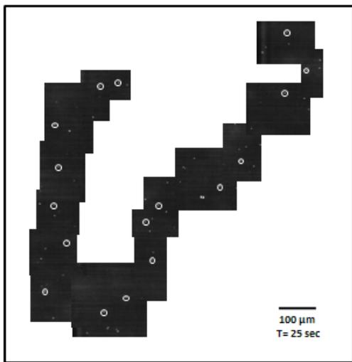
Figure 7. Mosaic image of the tracking of a bacterium on few millimeters distance without magnetic control showing the random motion of the MC-1
