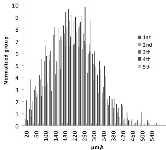
Figure 8. Normalized speed distribution for five different MC-1 under magnetic control.
