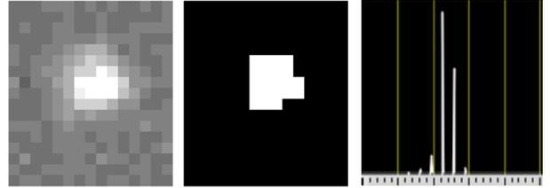
Figure 5. Otsu Segmentation Method applied to a bacterium. Left a bacterium capture with the CCD, center the same bacterium after Otsu segmentation, right the intensity histogram of the original image.
