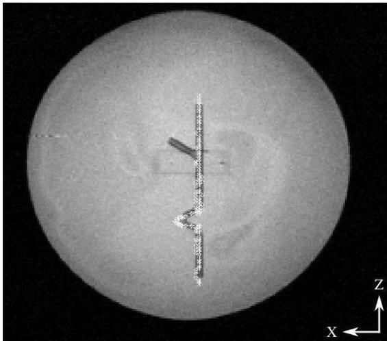
Figure 10: Result of the tracking in the glass phantom in a spherical aquarium. The dots represent the catheter tracked points as viewed in the fiducials module of 3DSlicer (medical imaging software). Axis added.
