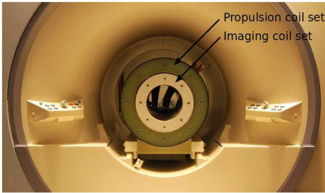
Figure 2: Magnetic gradient coil sets inside the bore of a 1.5T Siemens Sonata MRI system - The outer cylinder is responsible of high amplitude and duty cycle gradients for propulsion. The inner cylinder provides high linearity and responsiveness gradients for imaging purpose.
