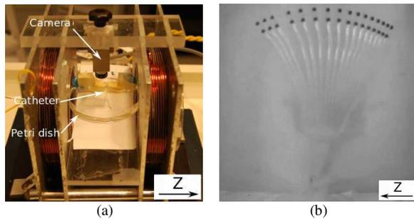
Figure 3: Comparison experiment: (a) shows the experimental setup; (b) is a superimposed picture of the deflections obtained by varying the gradient amplitude by 50mT/m increments from -400mT/m to +400mT/m.
