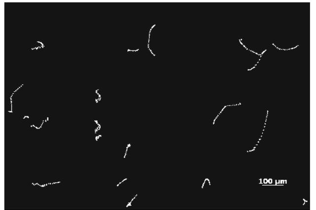
Fig. 3. Binary reconstruction of a time-lapse stack of 40 segmented and OR<sup>ed</sup> *S-images*.
