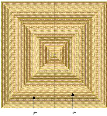
Fig. 4. View of the architecture of the cell from Cadence layout Virtuoso.
