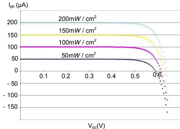
Fig. 5. Simulated I-V characteristics of the photocell for different green light intensities [9].
