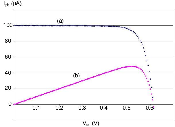
Fig. 6. (a) Simulated I-V characteristics of the photocell for 100mW/cm<sup>2</sup> green light intensity. (b) Simulated P-V characteristics of the photocell for different light intensities [9].
