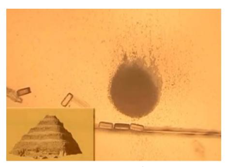
Researchers at the <u>NanoRobotics Laboratory</u> of the École Polytechnique de Montréal, in Canada, are putting swarms of bacteria to work, using them to perform micro-manipulations and even propel microrobots.
