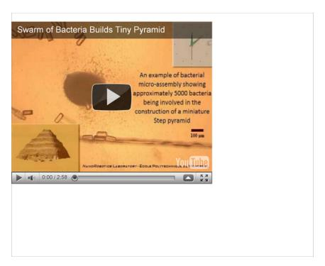
The bacteria, of a type known as magnetotactic, contain structures called magnetosomes, which function as a compass. In the presence of a magnetic field, the magnetosomes induce a torque on the bacteria, making them swim according to the direction of the field. Place a magnetic field pointing right and the bacteria will move right. Switch the field to point left and the bacteria will follow suit.
