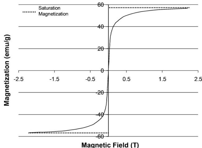
FIG. 1. Magnetization curve of Fe<sub>3</sub>O<sub>4</sub> magnetic suspension.
