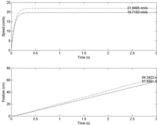
Fig. 2 Position and speed vs time for an open-loop simulation
