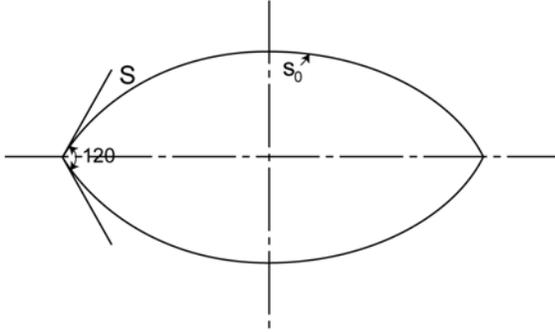
Fig. 1 Prolate spheroid with smallest drag in Stokes flow
