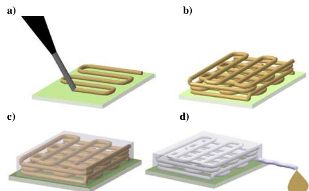
**Figure 1:** Schematic illustration of the fabrication process for 3D microchannel networks by direct ink writing: a) deposition of the ink through micronozzle; b) layer-by-layer ink deposition; c) epoxy infiltration of network; d) epoxy solidification and removal of fugitive ink.
