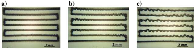
**Figure 2:** Depositions of  $200\mu\text{m}$  of hydraulic diameter ink patterns using the Fisnar J2200 apparatus. Depositions made at the constant speed of (a)  $10\text{mm/s}$ , (b)  $20\text{mm/s}$  and (c)  $30\text{mm/s}$ .
