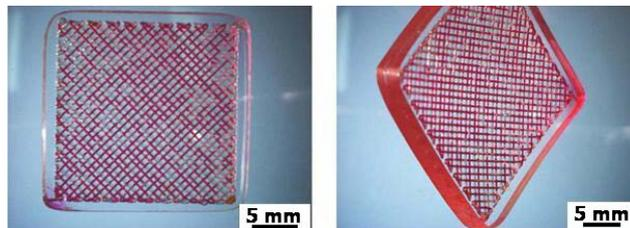
**Figure 12:** Top (a) and isometric (b) views of a 2 layer microchannel network (250µm of diameter) filled with a colored fluid.
