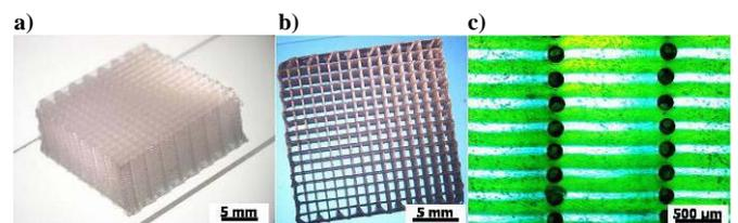
**Figure 10:** Isometric (a) and top (b) view of a 54-layer scaffold made of binary organic ink (20 wt-% microcrystalline wax) deposited through a  $200\mu\text{m}$  nozzle at a speed of  $88\text{mm/s}$ . c) Scaffold filled with a fluorescent fluid after an epoxy infiltration and the removing of the fugitive ink.
