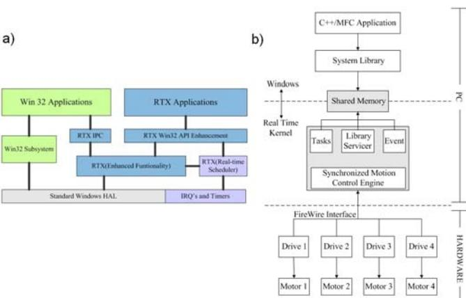
**Figure 4:** a) RTX software diagram. The hardware abstraction layer (HAL) of RTX provides resources for a real-time clock (shortest period of 100  $\mu$ s) and an insulation of the interruptions set by RTX over layers. The Real-Time SubSystem (RTSS), which provides the functions and resources management, is simply a hardware driver installed on Windows. b) Positioning system hardware/software simplified diagram.
