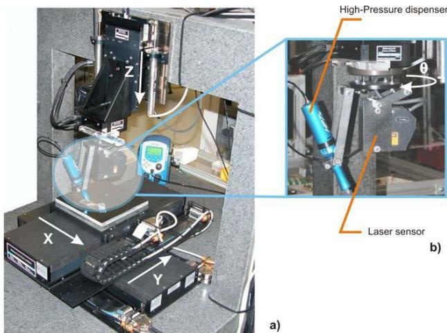
**Figure 3:** a) Complete experimental setup with four displacement axes placed in gantry configuration, granite structure, air dispenser, mechanical valve and the syringe. The two horizontal displacement robots (ALS25000, Aerotech) place in Cartesian configuration. b) The rotary stage (ADRS150, Aerotech) mounted under the vertical stage (AIS130, Aerotech) in a cylindrical configuration.
