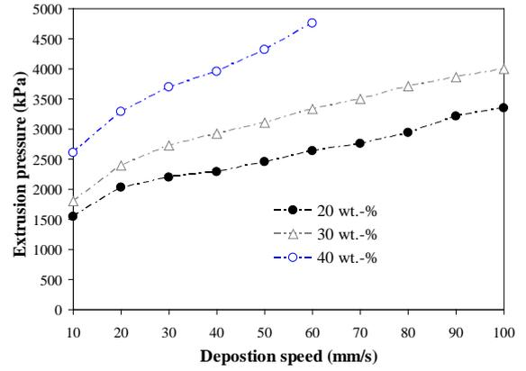
**Figure 6:** Extrusion pressure required to maintain a 200 $\mu$ m ink diameter during the deposition for inks containing 20% and 40% of microcrystalline wax.
