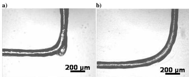
**Figure 8:** a) 90-degree corner written with a  $100\mu\text{m}$  filament. b) Smoothened corner using B-Spline algorithm written with a  $100\mu\text{m}$  filament.
