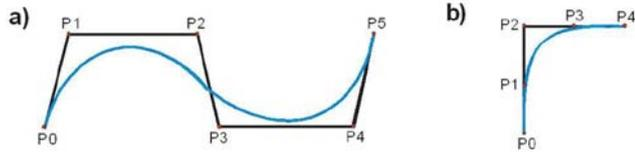
**Figure 5:** a) B-Spline curve. b) Isolation of a corner using the B-Spline algorithm.
