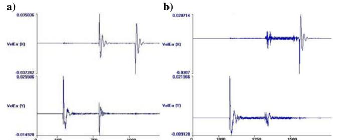
**Figure 9:** X and Y (horizontal displacements stage) velocity error  $\text{inmm/s}$  versus time in ms during the deposition of a a) 90-degree turn written with a  $100\mu\text{m}$  filament. b) Smoothened 90-degree turn using a B-Spline algorithm written with a  $100\mu\text{m}$  filament.
