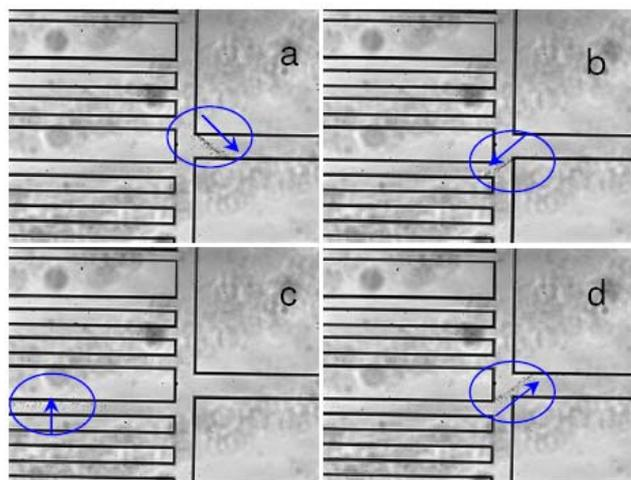
Fig. 5 A group of MC-1 MTB is manipulated in microfluidic channels by re-orienting the direction of a 10 Gauss magnetic field.
