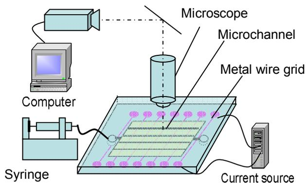
Fig. 4 Experimental setup for observing and recording the activity of MTB in the microchannels.
