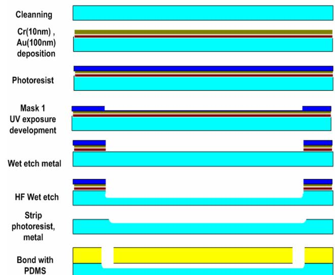
Fig. 3 Microfabrication procedure for the microchannels.
