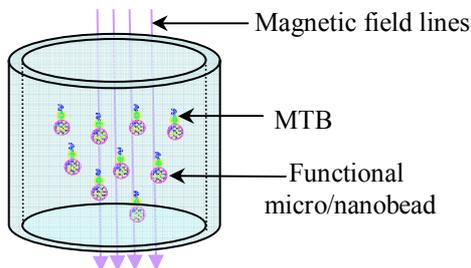
Fig. 2 Schematic representing the MTB transporting the functional micro/nanobeads under the control of a directional magnetic field.
