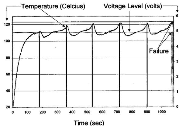
Figure 3. Experimental data for the 1.22mm thick water boiling convection jacket at 13.5W power dissipation with 0.6 gram refill every 3 minutes.
