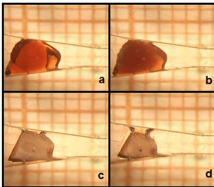
Fig. 5. Remarkable volume reduction (a-d) of 20 mm<sup>3</sup> 5 mgFe/ml NIPA hydrogel when heated to 29 °C to less than 12 mm<sup>3</sup>.
