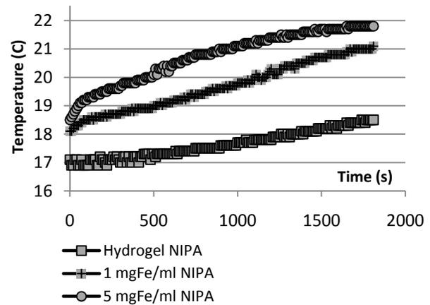
Fig. 6. Temperature change versus time for two samples of hydrogel embedded MNP inside *Agar gel* and hydrogel control sample.
