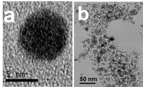
Fig. 1a. TEM image of a single domain Iron Oxide MNP
