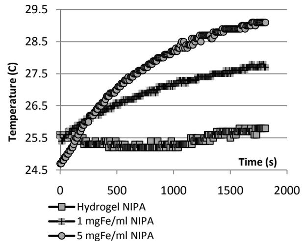
Fig. 7. Temperature change versus time for two samples of hydrogel embedded MNP inside *styrofoam insulation* and hydrogel control sample.
