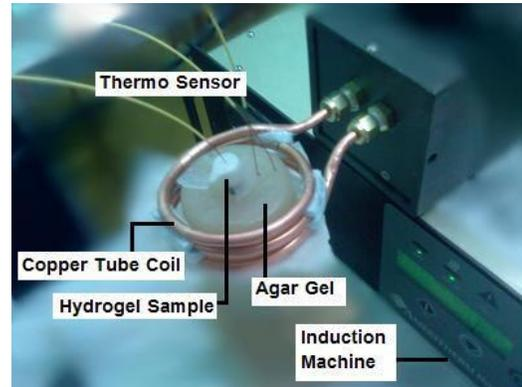
Fig. 3. Induction of hydrogel sample in Agar gel.
