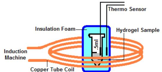
Fig. 4. Schematics of induction of hydrogel sample in insulation styrofoam.
