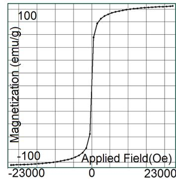
Fig. 2. Lack of hysteresis curve of MNP obtained by VSM measurements indicates superparamagnetic behavior of our Iron Oxide MNP.
