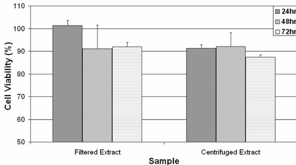
Fig 4. L-929 viability after exposure to  $Tb_{0.27}Dy_{0.73}Fe_{1.95}$  powder.
