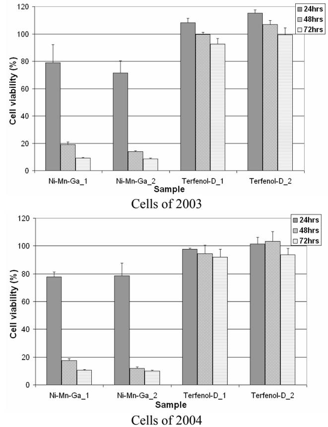
Fig 2. L-929 (2003) viability after exposure to single crystal Ni-Mn-Ga powder (Ni-Mn-Ga\_1 & Ni-Mn-Ga\_2) and  $Tb_{0.27}Dy_{0.73}Fe_{1.95}$  samples (Terfenol-D\_1 = sample 1 & Terfenol-D\_2 = sample 2).
