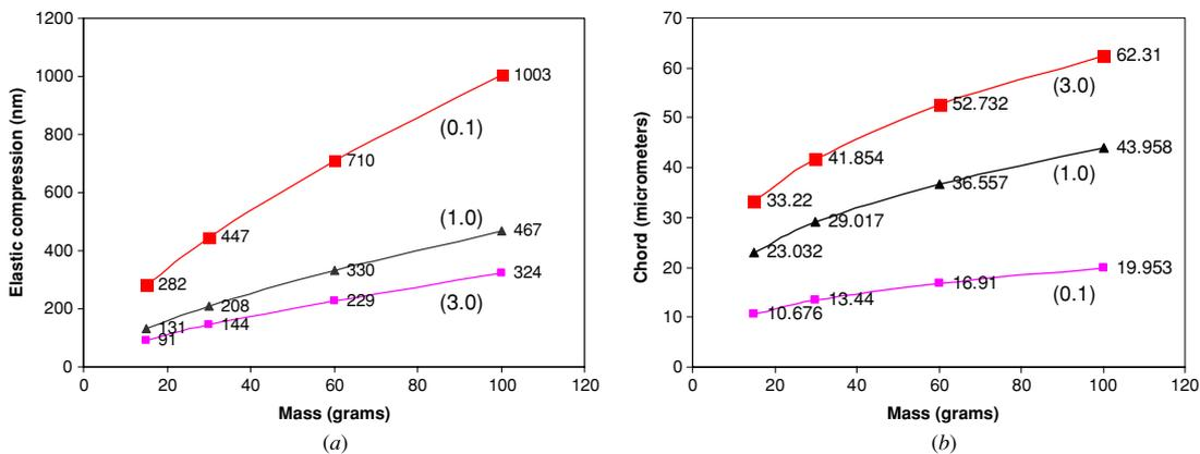
**Figure 6.** (a) Estimation of the elastic compression versus the total mass of the three-legged robot at 25 °C between a single leg and the insulating band with  $D_F = 3.0, 1.0$  and  $0.1$  mm and (b) resulting chord length  $R$ . The results assume a perfectly flat surface.
