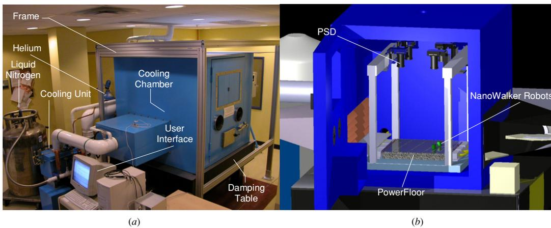
**Figure 3.** Implementation of the nanorobotics platform designed to accommodate a fleet of at least 100 NanoWalker robots: (a) photograph of the platform with the cooling chamber and (b) showing a CAD representation of the PowerFloor and other main components inside the cooling chamber.
