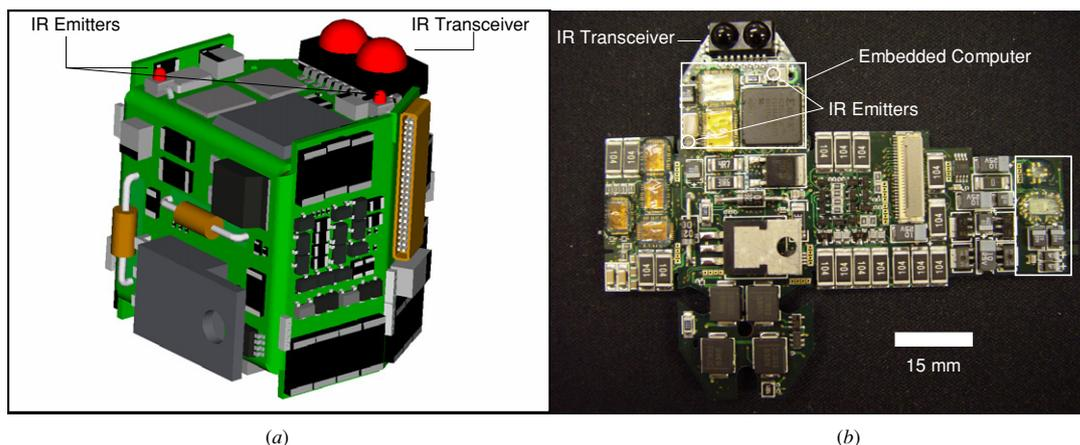
**Figure 4.** (a) CAD-based representation of the NanoWalker robot showing the IR emitters and IR transceiver on top and (b) a photograph of the upper side (lower side not shown) of the multilayer circuit unfolded showing the position of the IR emitters and IR transceiver.
