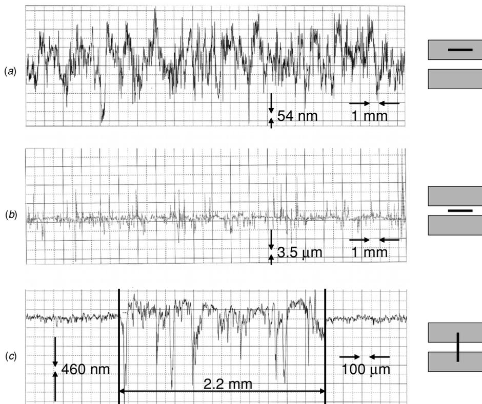
**Figure 7.** Flatness of the surface of the PowerFloor measured with a profilometer: (a) along the longitudinal axis of a 440C stainless steel conducting band, (b) along the longitudinal axis of a back granite insulation band and (c) along the transversal axis between two conducting bands.
