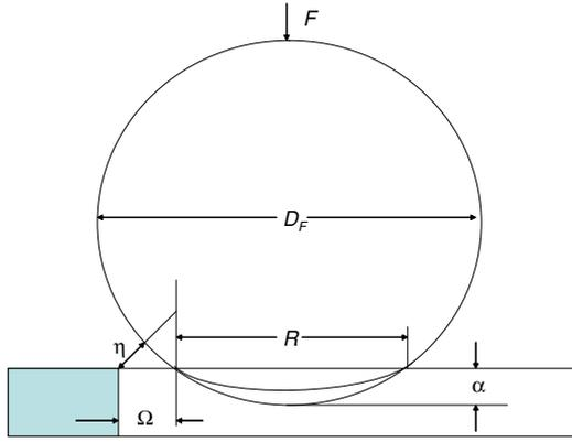
**Figure 5.** Basic model of the extremity of a leg (foot) on the insulating band of the PowerFloor. The shadowed region represents a conductive band.  $F$ ,  $R$ ,  $\eta$  and  $\alpha$  represent the force acting on the foot, the chord of the surface contact, the minimum distance to prevent arcing and the elastic compression, respectively.
