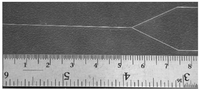
Fig. 6. Y-shaped microvascular channel fabricated by direct write assembly
