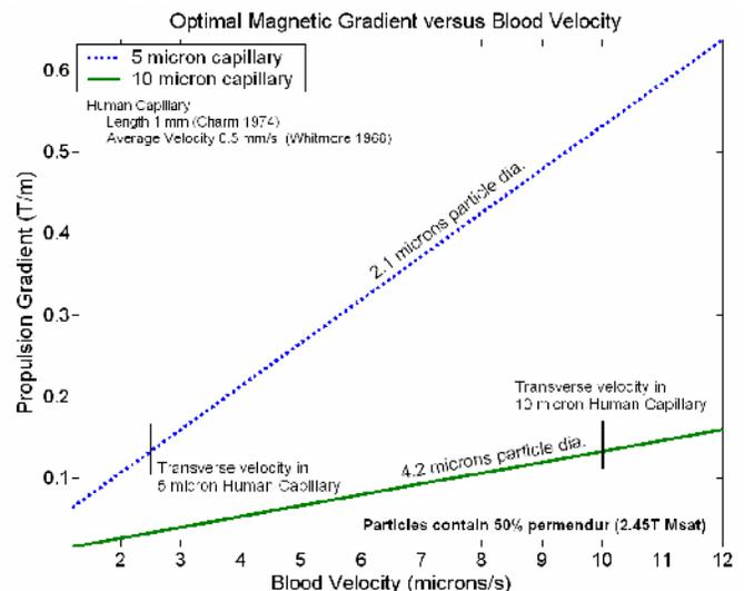
Fig. 2. Steering gradients for 2.1 and 4.2 micrometer diameter 50% volume Permendur sphere in human capillaries with diameters of 5 and 10 micrometers (physiological specifications from [3]). According to the steering criterion, approximately 100 mT/m gradients are required for steering of 2.1 and 4.2 micron particles in such capillaries.
