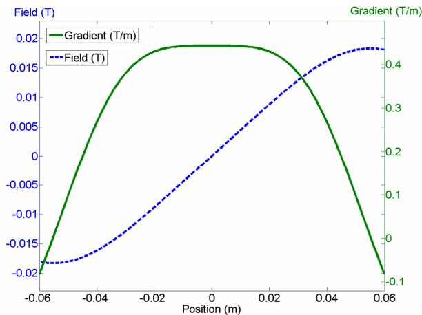
Fig. 5. Magnetic field and gradient of the Maxwell pair ( $I=20A$ )
