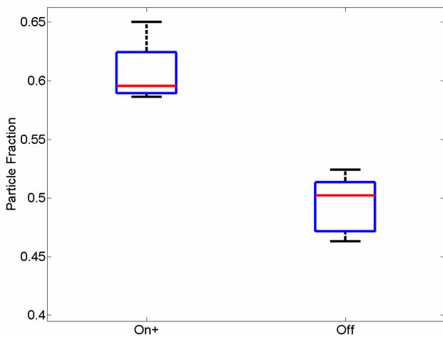
Figure 7. Box plot of the ratio of particles at the positive outlet. The ‘On+’ box shows the particle fraction when the gradient coil is applied (average = 0.61), the ‘Off’ box shows the particle fraction when the gradient coil is not applied (average = 0.48).
