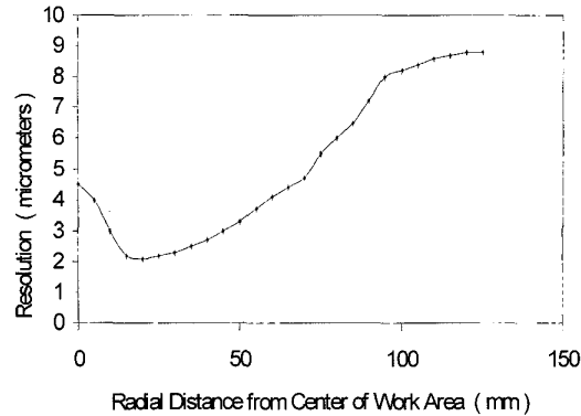
Fig. 8. Resolution of the PSD-based System (from [16])
