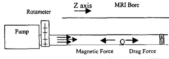
Fig. 1. MRI propulsion set-up for experiment 1
