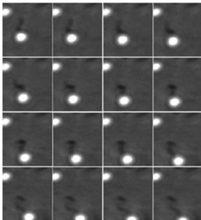
FIG. 3. Close-up view of a microbead being pushed by a single MTB.
