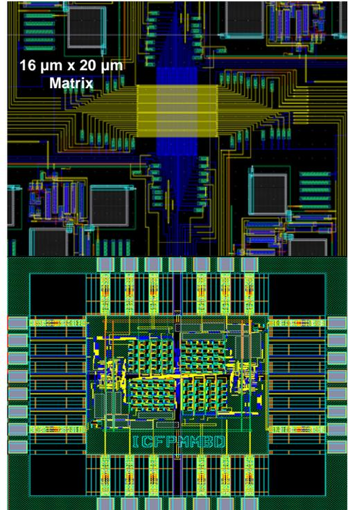
Fig.4 Matrix layout in Cadence
