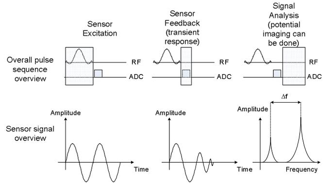
Figure 1: Overview of the functionality and MRI sequence for the sensor operation and data analysis.
