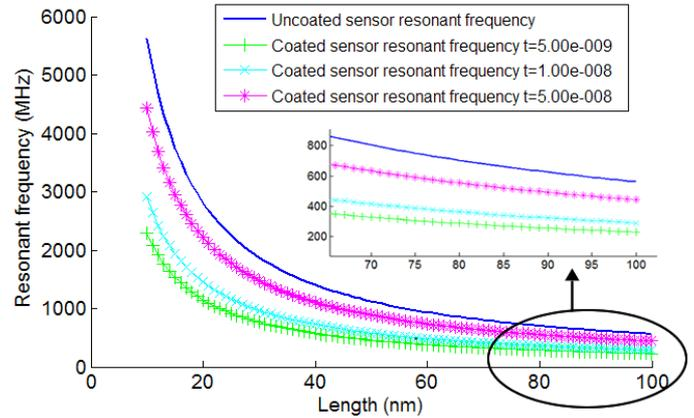
Figure 2: Resonant frequency of a uncoated and pH polymer coated magnetoelastic material in function of the selected length of the sample
