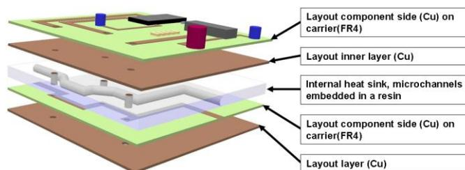
Fig. 2. Exploded view of a four layer PCB with an embedded microchannel.
