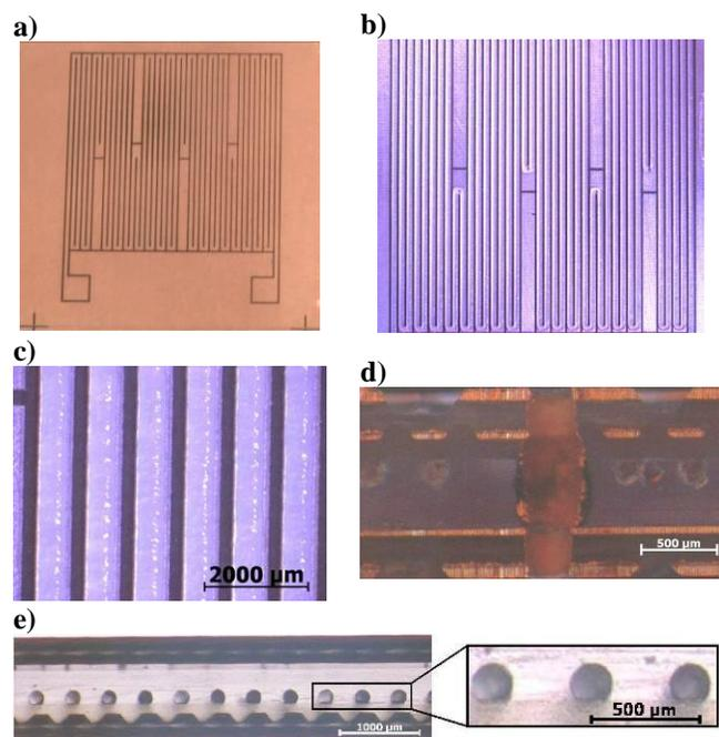
Fig. 3. a) Internal copper layout used for microfabrication and thermal testing of micro heat exchanger; b) Ink pattern deposited over copper trace following circuit drawings ( $500$   $\mu\text{m}$  filament diameter); c) Larger view of ink the filaments over the layout; d) Electroplating of a via of  $300$   $\mu\text{m}$  of diameter on a resin/FR4/copper sheet; e) Side view of  $200$   $\mu\text{m}$  of diameter channels embedded between two FR4/copper sheets.
