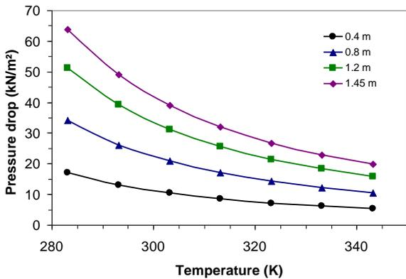
Fig. 7. Calculated pressure drop versus the average fluid temperature for different microchannel length (coolant fluid: water, flow rate = 3ml/min).
