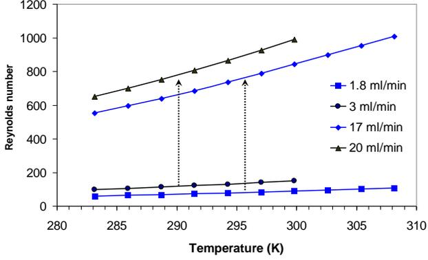
Fig. 6. Calculated Reynolds number versus the average fluid temperature in a 500  $\mu\text{m}$  diameter channel for a flow rate of 1.8ml/min ( $\Delta$  25 K) and 3ml/min ( $\Delta$  15 K) and their extrapolation at the maximum flow rate prior to turbulent behavior.
