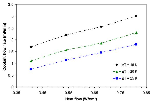
Fig. 5. Experimental results of water flow rates needed to dissipate heat flux for different temperature gradients in a 500  $\mu\text{m}$  diameter channel.
