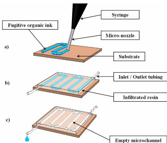
Fig. 1. Schematic representation of the fabrication process of a two dimensional microchannel by direct-write assembly: a) Extrusion of ink through a micro-nozzle and robotic deposition on substrate; b) Fluidic connection and epoxy infiltration; c) epoxy solidification and removal of fugitive organic ink.
