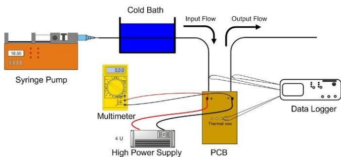
Fig. 4. Schematic representation of the thermal setup used to characterize the thermal efficiency.
