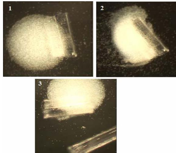
**Fig. 4:** A population of MC-1 bacteria pushing a larger object under directional control for the implementation of a more powerful robot (approximately 5000 MC-1 cells have been used in this specific example).
