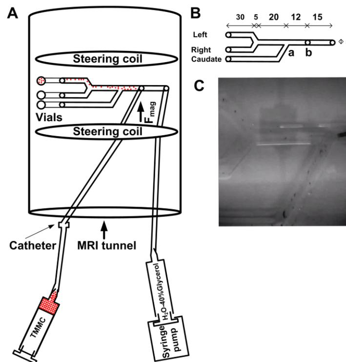
**Fig. S3:** *In vitro* steering MRI setup. Image A represents a schematic view of the MRI steering setup. Image B is a schematic view of the hepatic artery phantom with its dimensions. On the image, a and b refer to the position of the catheter tip. Image C displays a frame extracted during the recording of a TMMC steering test when the catheter was placed at 20 mm from the bifurcation.
