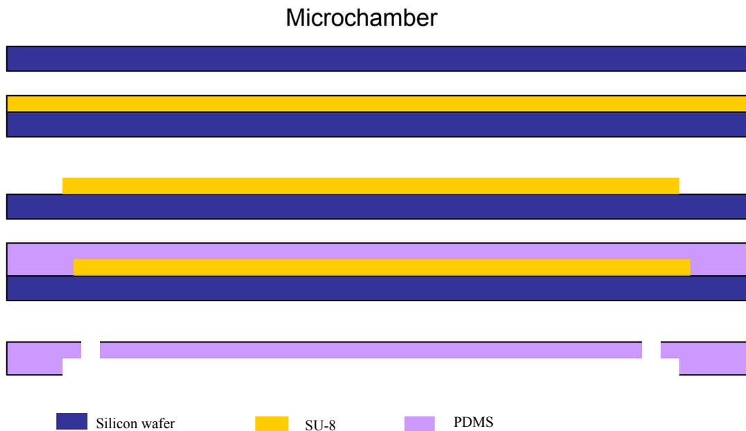
Fig. 6. Fabrication steps of (a) microelectromagnets and (b) microfluidic sections.
