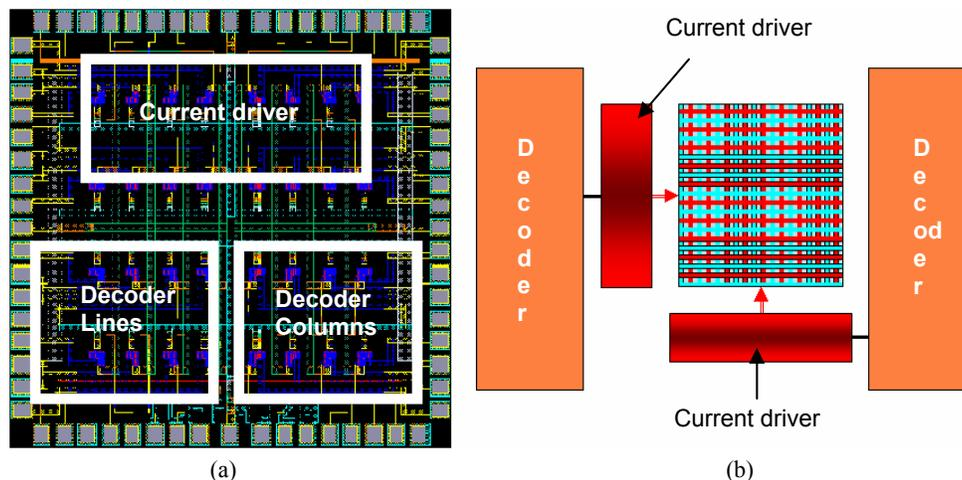
Fig. 2. Internal architecture of the microelectronic chip
