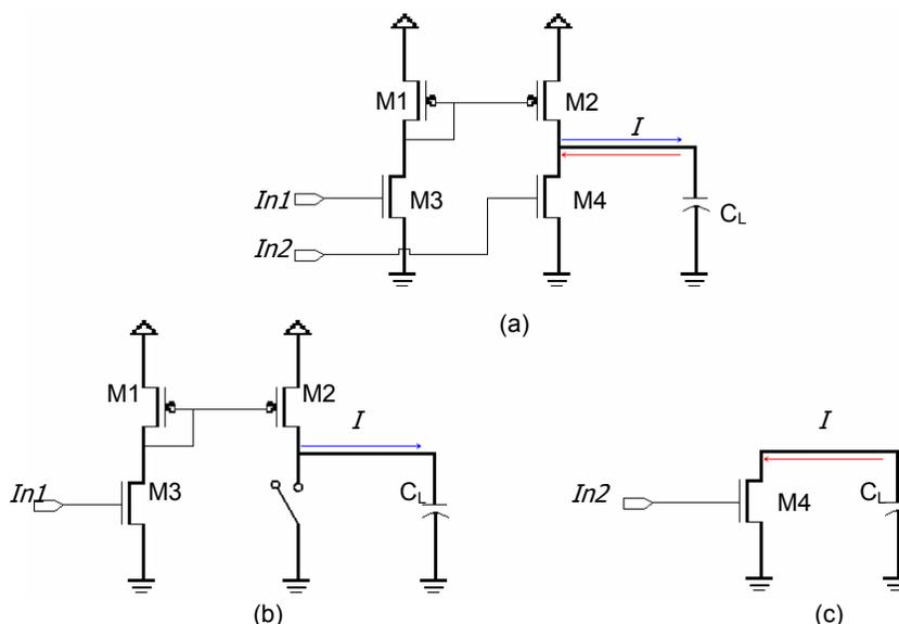
Fig. 3. (a) Circuit for the current driver to generate the magnetic field to navigate the bacteria. (b) Shows the current flowing into one direction for a particular motion of the MTB (c) shows the reverse direction of the current; therefore reverses the direction of the magnetic field.
