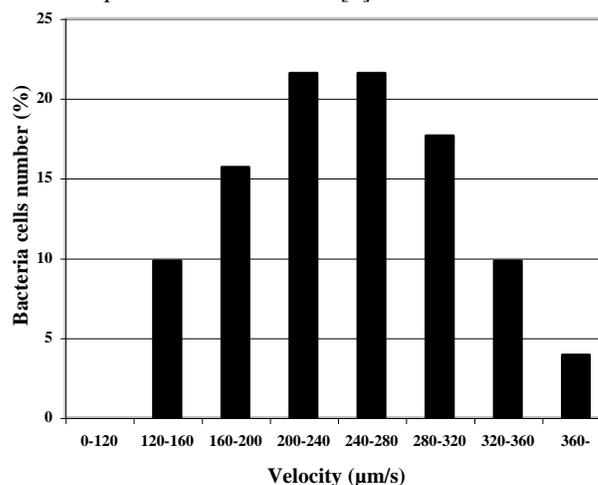
*Figure 3: Swimming speed Distribution of MC-1 when cultivated in  $55\mu\text{Mol}$  of ferrous sulfate ( $\text{FeSO}_4$ ). Cells were suspended in PBS buffer.*
