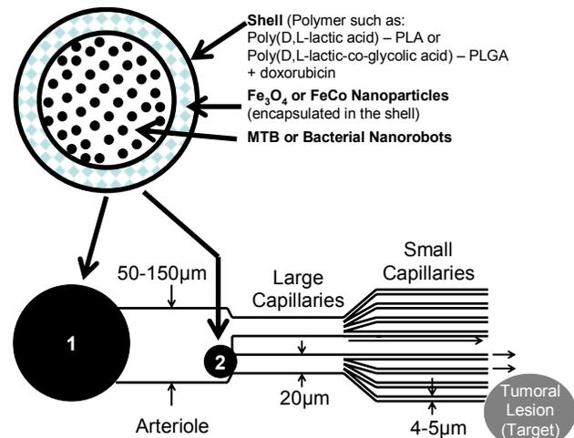
Fig. 1. Diagram of a micro-carrier with the two target embolization sites denoted as 1 and 2 in black circles where MTB-tagged nanorobots can be released. Release at the arteriole entry (site 1) is possible with a clinical MRI platform upgraded with software only whereas release at the arteriolar entry (site 2) for enhanced targeting efficacy is possible by upgrading existing MRI machine with coils capable of higher magnetic gradients.
