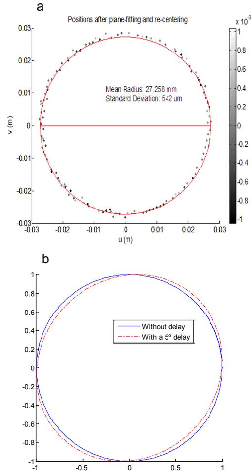
Fig. 5. (a) Positions after plane fitting and re-centering. The gray-scaled dots indicate the distance perpendicular to the plane. (b) Simulation of the delay between the  $x$  and  $y$  acquisitions.
