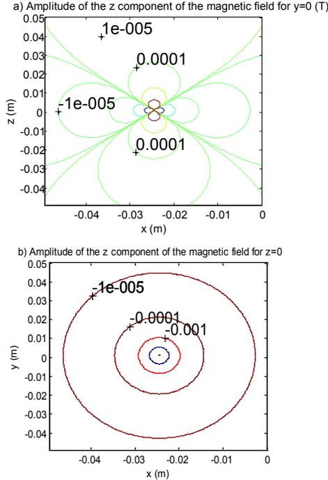
Fig. 1. Simulation of the magnetic field (T) generated from a 1mm diameter ferromagnetic bead ( $B_{sat} = 1.67T$ ) in a 1.5T surrounding field. a) Sagittal or coronal cut with  $y=0$ ; b) axial cut with  $z=0$ . The MRI static field is along  $z$ .
