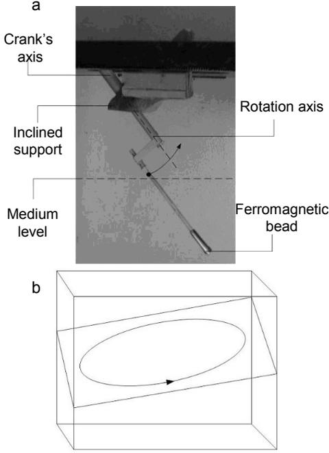
Fig. 3. (a) Photograph of the mechanical setup used to obtain a displacement along a precise 3D circle. An illustration of the circular motion is given in (b).
