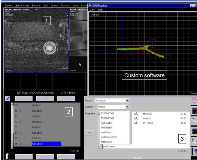
Fig. 6. User interface showing our custom software projecting the position of the bead in real-time along the pre-planned path. Numbered boxes refer to the Siemens user interface. In (1) it is shown an off-resonance image acquired to tune up the tracking sequence parameters. (2) shows the current running sequence and (3), the Siemens sequence explorer interface
