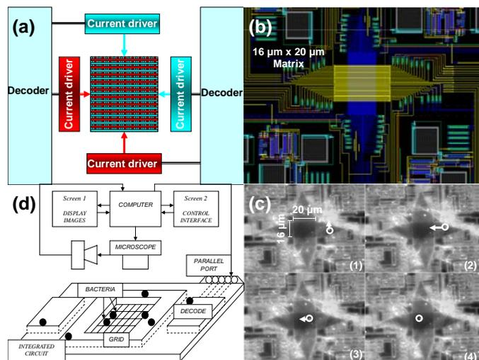
Fig. 3. (a) Bloc diagram of the hardware architecture; (b) Matrix layout as shown by the Computer-Aided Design (CAD) software; (c) Influence of the magnetic field on the bacterium's trajectory; (d) General overview of the platform.
