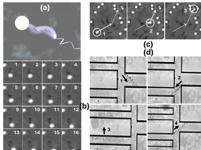
Fig. 1. (a) Basic concept of the bacterial carrier or microrobot; (b) Closed-up view of the real implementation using a  $3 \mu\text{m}$  diameter bead showing the displacement of the microrobot in an aqueous solution; (c) Example of navigational control of a single bacterial microrobot; (d) Navigational control of a swarm of magnetotactic bacteria in microfluidic channels observed under an optical microscope.
