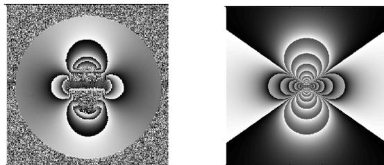
Fig. 2. Magnetic dipole MRI phase image (left) and simulated field mapping (right) of a 1010/1020 carbon steel sphere (from [5]).
