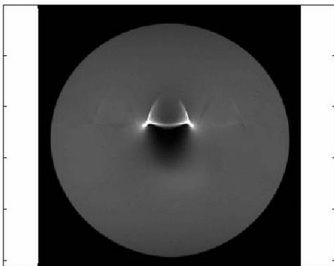
Fig. 1. MRI image artifact of a 1010/1020 carbon steel sphere.
