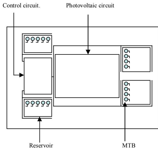
Fig. 1. Schematic (not to scale) of the global architecture of the ABS with an overall estimated size of  $500 \mu\text{m} \times 200 \mu\text{m}$ .
