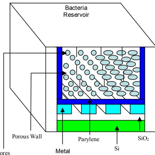
Fig. 3. Cross-section of a reservoir containing the MTB and acting as a "bacterial engine". Directional control is assured by inducing a torque on the chain of magnetosomes embedded in each bacterium by passing an electrical current in the metal conductors.
