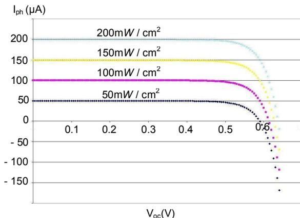
Fig. 5. Simulated I-V characteristics of the photocell for different green light intensities [9].
