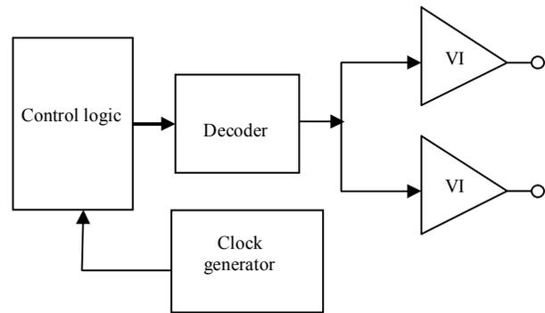
Fig. 2. Schematic of the internal architecture of the microelectronics embedded in each ABS. VI stands for voltage to current converter.
