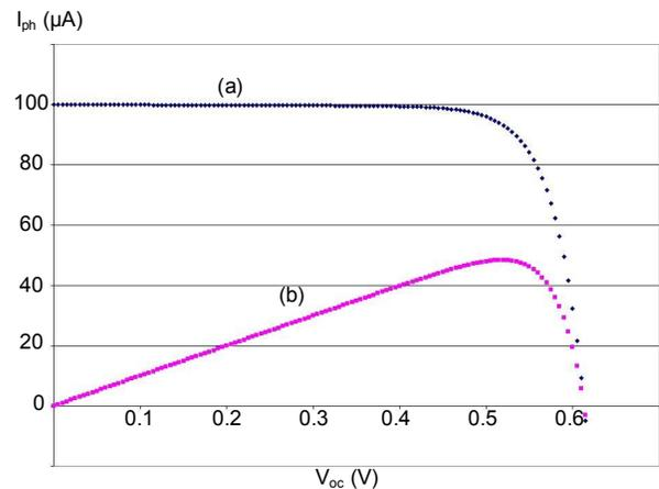
Fig. 6. (a) Simulated I-V characteristics of the photocell for 100  $\text{mW}/\text{cm}^2$  green light intensity. (b) Simulated P-V characteristics of the photocell for different light intensities [9].
