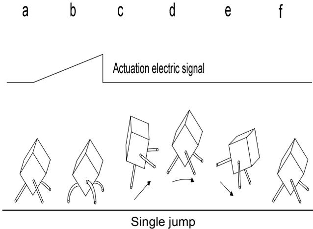
Fig. 7 Basic principle of locomotion, a. initial position, b. combined forces from the legs and the floor, c. robot is lifted, d. robot losing contact with the floor, e. robot is falling down, f. robot is back on the floor. The deflection amplitudes of the legs are exaggerated here for clarity.
