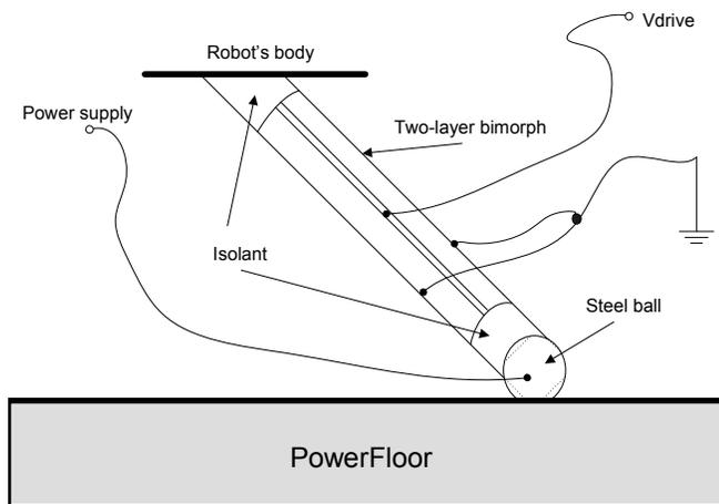
Fig. 2 Schematic of one actuating leg
