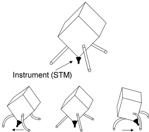
Fig. 8 Simplified schematics showing the scanning operations. Again, the amplitudes of deflection of the legs have been exaggerated here for clarity.
