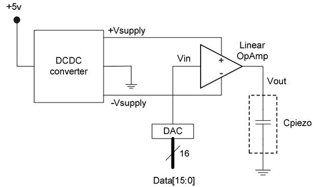
Fig. 9 Simplified block diagram showing the main driving circuit
