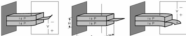
Fig. 6 Two-layer bending element poled for parallel operation (from [4]).
