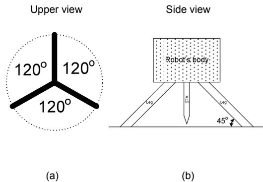
Fig. 4 Geometry of the actuation system embedded in each robot, (a) upper view and (b) side view
