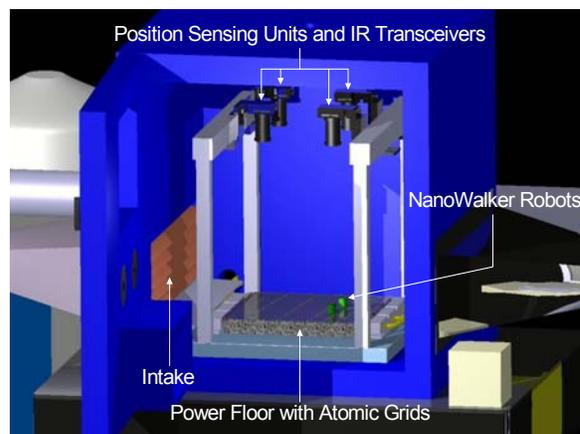
**Figure 8. Inside the cooling chamber**
