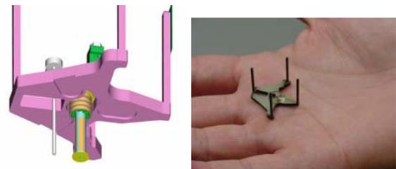
**Figure 1. Representation of the STM tip encapsulated in the robot's skeleton with a photograph of the skeleton in a hand**
