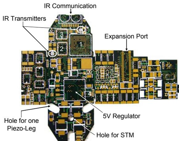
**Figure 6. Photograph of the bare board**
