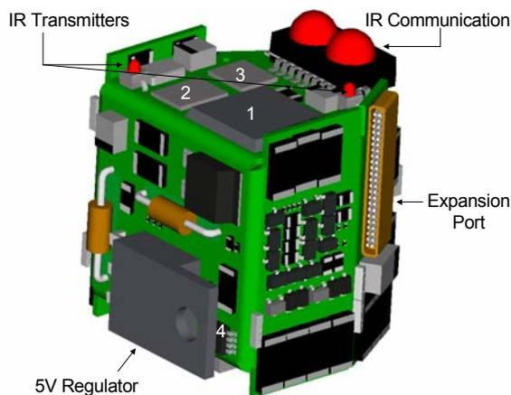
**Figure 5. View of the NanoWalker robot**
