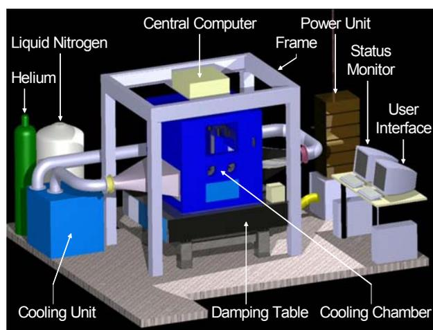
**Figure 7. CAD representation of the cooling platform**
