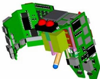
**Figure 3. CAD representation showing the flexible circuit architecture**
