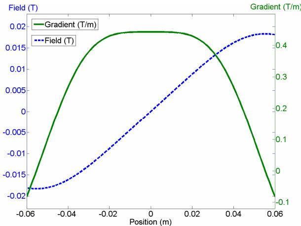
Fig. 5. Magnetic field and gradient of the Maxwell pair ( $I=20\text{A}$ )
