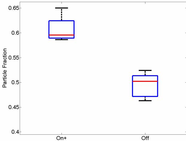
Figure 7. Box plot of the ratio of particles at the positive outlet. The ‘On+’ box shows the particle fraction when the gradient coil is applied (average = 0.61), the ‘Off’ box shows the particle fraction when the gradient coil is not applied (average = 0.48).
