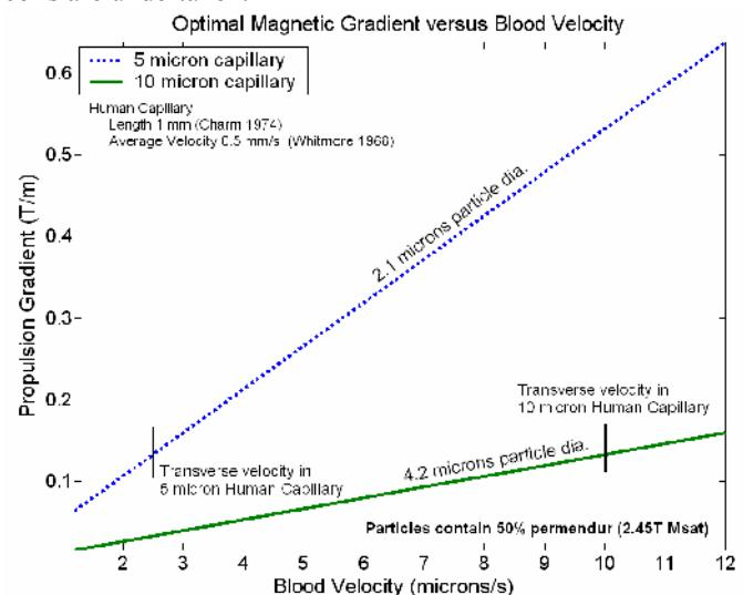
Fig. 2. Steering gradients for 2.1 and 4.2 micrometer diameter 50% volume Permendur sphere in human capillaries with diameters of 5 and 10 micrometers (physiological specifications from [3]). According to the steering criterion, approximately 100 mT/m gradients are required for steering of 2.1 and 4.2 micrometers in such capillaries.
