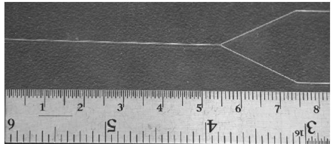
Fig. 6. Y-shaped microvascular channel fabricated by direct write assembly
