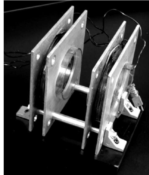
Fig. 4. Photograph of the Maxwell pair developed for the experiments
