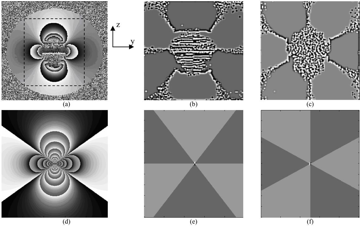
Fig.1. Magnetic dipole MRI phase image and gradient calculation; (a) Experimental field mapping of 1010/1020 carbon steel sphere, (b) Spatial gradient of experimental field mapping along the z direction, (c) Spatial gradient of experimental field mapping along the y direction, (d) Simulated field mapping of 1010/1020 carbon steel sphere, (e) Spatial gradient of simulated field mapping along the z direction, (f) spatial gradient of experimental field mapping along the y direction.
