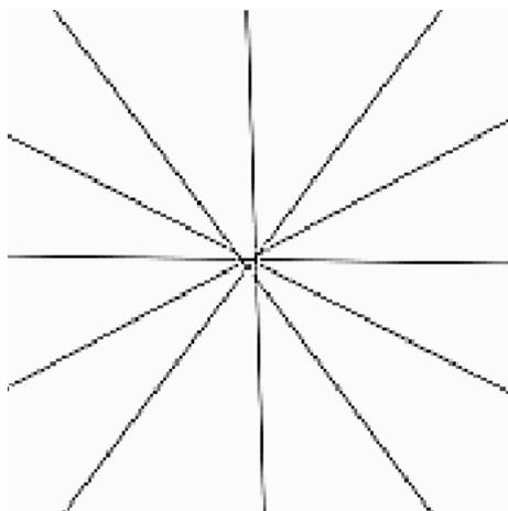
Fig. 2. Intersection lines of the change in sign of the magnetic gradient of the phase image. The convergence of the lines indicates the position of the dipole
