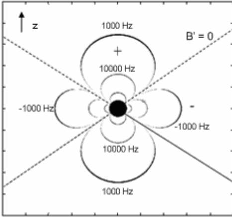
Fig. 1. MATLAB Simulation of the spatial distributions of the resonant frequency.
